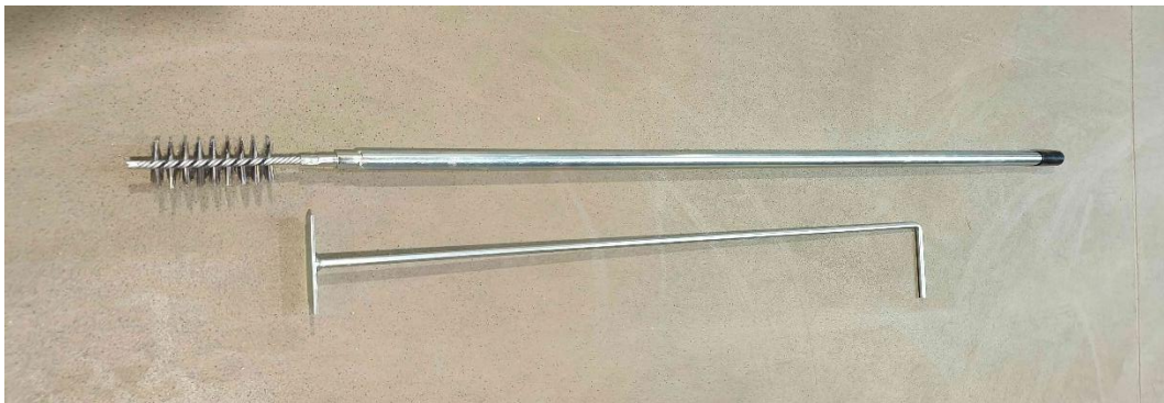
Figure 24. Cleaning tools for the RPC boiler
