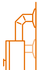
CHIMNEY CONNECTION (FROM ABOVE OR BEHIND)
